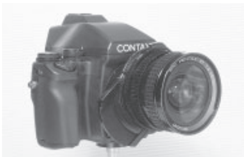
Pro Shift Adapter (ProSA-P67) with 45 mm Pentax 67 lens
